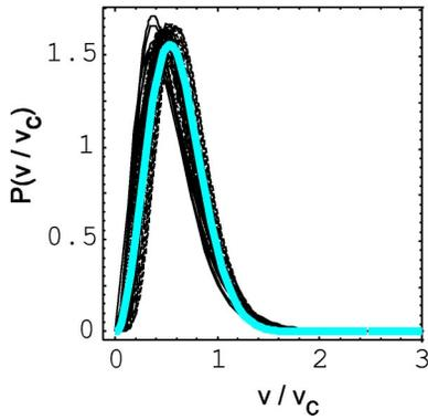
FIG. 7. Dark lines are the scaled speed-dependent transmission  $T(v)$  of  $^{85}\text{Rb}$ ,  $^{87}\text{Rb}$ ,  $^6\text{Li}$ ,  $^7\text{Li}$ ,  $^{133}\text{Cs}$ , and  $\text{S}_2$  with  $K = 3, 9, 15, 21, 27, 33$  at bend ratios ranging from  $\gamma = 0.02$  to  $\gamma = 0.32$ , and fields ranging from  $B_w = 750$  G to  $B_w = 9000$  G. The light line is the Maxwell-Boltzmann speed distribution at the temperature  $T_{\text{eff}}$  given by Eq. (21).
