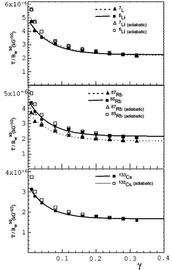
FIG. 4. Transmission of Li, Rb, and Cs atoms divided by  $B_w^{3/2}$ . Solid squares and triangles are the simulated transmission. Heavy solid and dotted lines are fits of the simulated transmission to guide the eye. Unfilled squares and triangles are simulated transmissions assuming only adiabatic motion.
