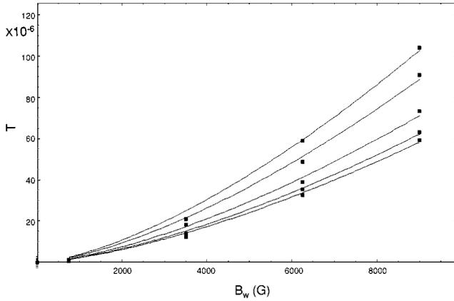
FIG. 3. Simulated transmission of  $^{85}\text{Rb}$  as a function of field strength  $B_w$  and  $\gamma = d/b_r$ , where  $d$  is the inner diameter and  $b_r$  is the bend radius of the filter. From the upper to the lower curve, the plots correspond respectively to  $\gamma$  of 0.04, 0.2, 0.12, 0.2, and 0.28. The points are the result of the Monte Carlo simulation, whereas the smooth lines are a fit to the points by the function  $T = \text{const}(B_w^{3/2})$ .
