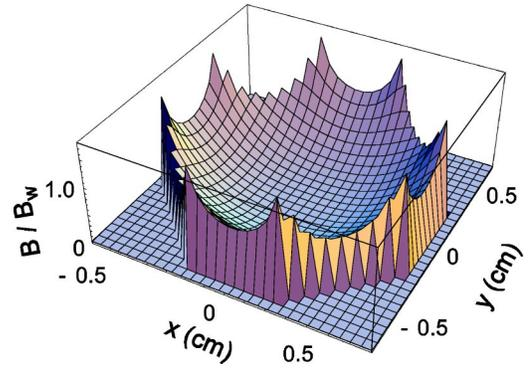
FIG. 2. Two-dimensional cross section of the magnitude of the magnetic field in a section of the guide, where  $B_w = \frac{1}{2}\mu_0 M$  is approximately the field at the face of each magnet and  $M$  is the magnetization.
