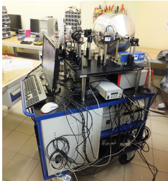
Fig. 3. Completely assembled device. In the upper right part of the device one can see the optical system of the device (schematically in Fig. 2). In the left part of the device there is a PC with a monitor, keyboard, and mouse to operate the device. In the bottom right part of the device one can find power supplies, laser control units, scan generators and the positioning table control unit. All of the devices which tend to vibrate are isolated with soft plastic materials. The device is placed on a cart with wheels, which allowed it to be moved about the lab.
